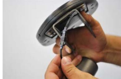
3. Feed the extra cable back into the handrail
