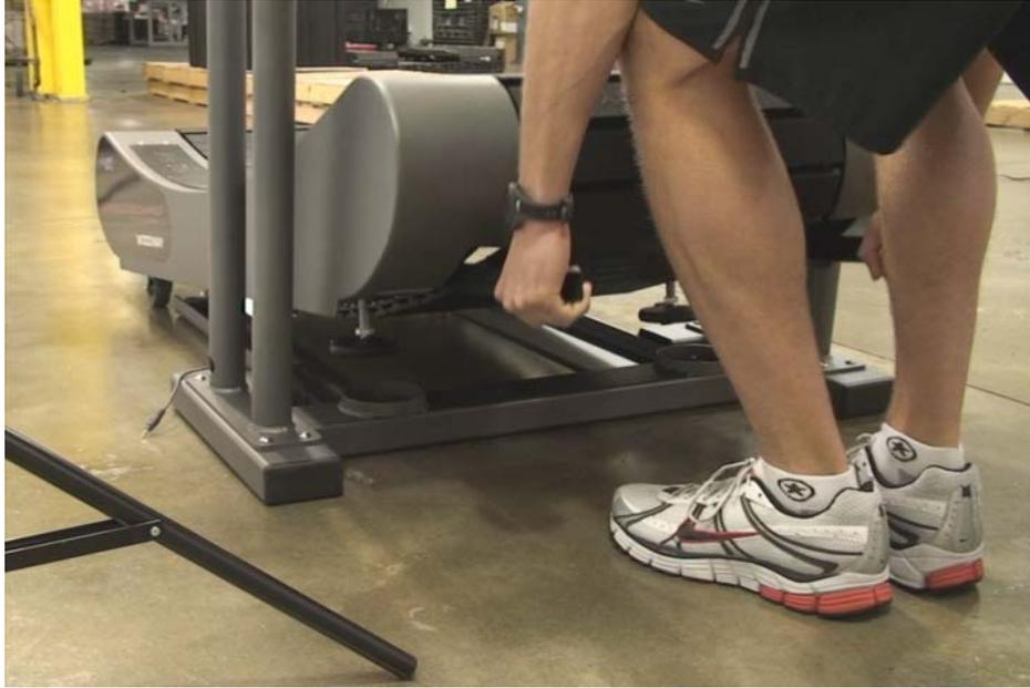
Lift the front of the treadmill and slowly wheel it onto the handrail base placing the front feet of the treadmill base into the 2 circle cups on the handrail assembly. The treadmill must be directly in line with the rail of the handrails assembly to assure proper installation.
