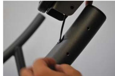
4. Line up the display on the handrail so that the 4 holes match up and the words are right side up for the user to read. Put the 4 allen head bolts into the four holes, be sure to put all four in loosely before tightening with the wrench.
