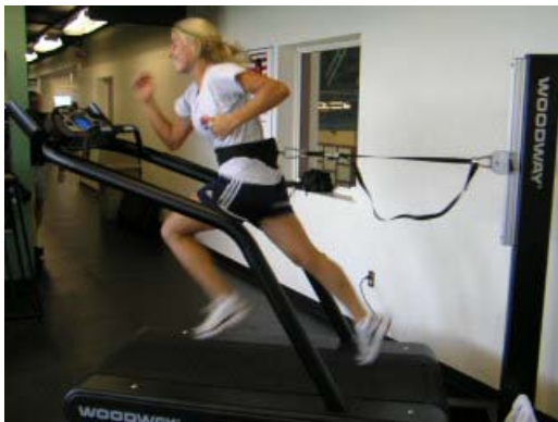
Figure 1: This graphic is of the Woodway Force Treadmill which uses a harness attached to a post behind the treadmill and a resisted belt system that allows the athlete to move the belt as opposed to a motorized system where the athlete simply has to keep up with the speed of the belt.
